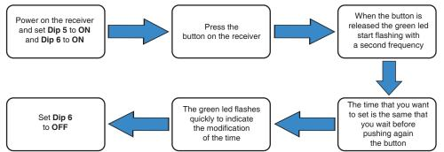
① For the timing of the contact of the output desired it must be set to timer mode (see paragraph 4).
